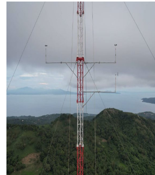
Anemometers and Wind Vanes at different levels (120, 100, 80, 60 meters)
