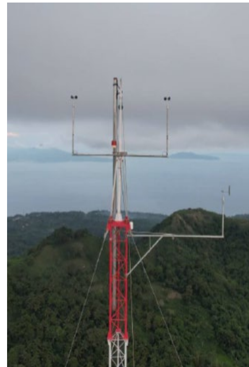
Anemometers and Wind Vanes at different levels (120, 100, 80, 60 meters)
